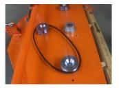
4. Place second belt over pulleys 2 and 3 fitting on highest groove
